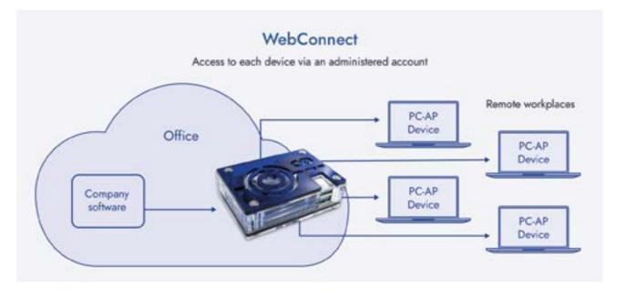
WebConnect gateway knows the devices that are to be accessible. Only between the gateway and the internal device is the remote connection established, which is then displayed and operated in the browser via HTTPS.
